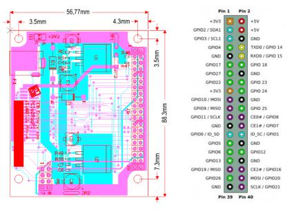
Obviously, FPGA can host a superset of Raspberry interfaces, on all the connector pins you can override the standard pin and set lot of different interfaces such as synchro, encoder, pwm, sio, spi, i2c, or also high-speed fifo. For instance, we can have 24xPWM channels or 8xPWM+ 8xI2C + 8xSPI.
