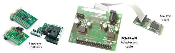
The PCIe2RasPI adapter routes the FPGA I/O pins to the standard Raspberry 40 ways J8 I/O connector, compatible A+, B+ and B2 versions. The peripherals that can be loaded on FPGA emulates the Raspberry Peripherals allowing the running of PC software under MS-Windows or Linux.
