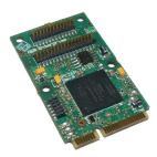
The standard Mini PCIe form factor is ideal for many kinds of applications; it is present on many compact PC motherboards such as Intel Galileo and Advantech MIO-5250
