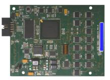
The default VME-IP and firmware support A32D32 master/slave cycles, interrupt handler, interrupter and SysCon. The related firmware (Monitor), running on NIOSII, allows the user to start all kind of bus cycles and some macro commands, such as memory test, using RS232 or USB data link.
